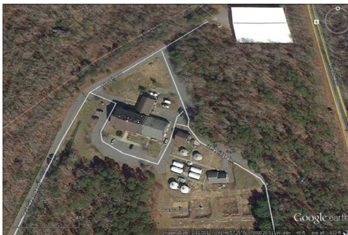
Rated for 45,000 gallons of septage per day (gpd), it was designed to thicken/condition/dewater septage solids prior to eventual shipment offsite. Liquid reject streams from these processes were collected and treated in a biological process consisting of rotating biological contactors (RBCs) prior to sedimentation, filtration, and ultimate discharge to rapid infiltration beds located on the site.
