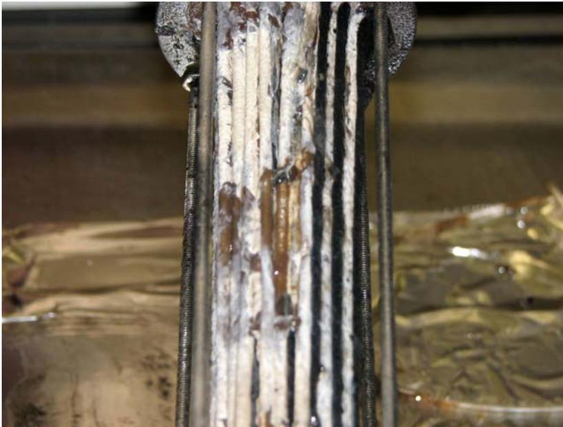
Figure 14. Picture of the RCB fiber module at harvest. Juxtaposed  $\text{H}_2$  (black) and  $\text{O}_2$  (white) fibers are clearly visible on the right portion of the module.
