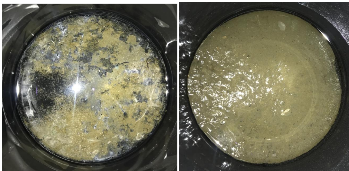
Figure VII.1 Images of sediment core surfaces from September 2017. Left: Core 3 within treatment area showed dark areas where reduced sediment was exposed to the water surface, thus preventing efficiently coupled nitrification and denitrification. Right: Core 13 outside of the treatment area showed a uniform oxidized surface.
